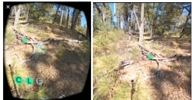
Figure 6: Joint session with instance on the left running in lead mode, while the instance on the right runs in follow mode. The left instance has just placed a circle marker on the ground that simultaneously appears in the instance on the right with arrows (not shown in the image) providing visual guidance.
