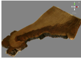
Figure 2: Photorealistic 3D model of a wood cookie from SfM.
